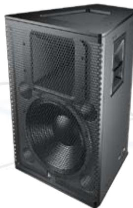
The UPQ-2P is a self-powered two-way loudspeaker designed for applications requiring high acoustic power output, extremely low distortion, and a narrow symmetrical coverage pattern with predictable characteristics. The UPQ-2P's compact, vented enclosure houses a 15-inch neodymium magnet low/mid driver, a 4-inch diaphragm compression driver coupled to a conical high frequency horn, and a two-channel amplifier with a total peak output power of 1275 watts. Maximum peak SPL measures 136 dB at 1 m.
