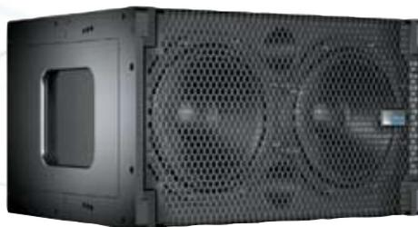
The dual 10-inch M1D-Sub ultracompact subwoofer features an operating frequency range of 32 Hz to 180 Hz. Designed specifically to work with the M1D ultracompact subwoofer, it extends overall system power bandwidth and frequency response to 35 Hz. The M1D-Sub produces 130 dB peak SPL at one meter from an extraordinarily small and light package, and employs a back-vented driver that features a two-inch voice coil with neodymium magnet and is rated to handle 400 AES watts.<sup>†</sup>
