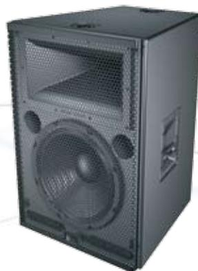
The CQ-2 narrow coverage main loudspeaker is a self-powered, phase-corrected reinforcement loudspeaker offering precise, high-Q coverage. The CQ-2 features a new, patented horn design that is the result of extensive research in Meyer Sound's calibrated anechoic chamber. The CQ-2's frequency response of 40 Hz to 16 kHz is uniform over the entire coverage area in both the horizontal and vertical axes, with no side lobes when measured at one-sixth octave frequency resolution.
