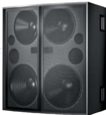
The PSW-6 high-power cardioid subwoofer is the first low-frequency system to exhibit a true cardioid directional pattern throughout its operating range. The PSW-6's unprecedented directional control spans more than two full octaves, with a front-to-back SPL ratio of more than 15 dB (typically 20 dB) from 30 Hz to 125 Hz. Horizontal and vertical coverage patterns are symmetrical, ensuring consistent SPL and frequency response throughout the coverage area.
