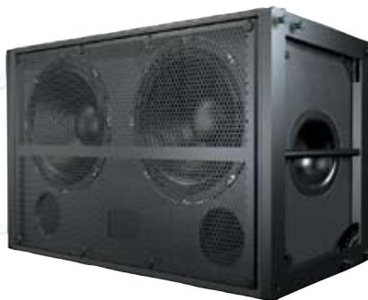
The dual 15-inch M2D-Sub compact subwoofer is designed to complement the M2D in reinforcement applications requiring extended low-frequency headroom, and features an operating frequency range of 28 Hz to 160 Hz. In combination with companion M2Ds, it extends the overall system power bandwidth and frequency response to 30 Hz.
