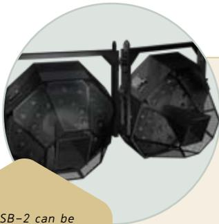
*The SB-2 can be suspended and aimed to provide wide-bandwidth sound in a tight 20-degree beam to a difficult coverage area.*
