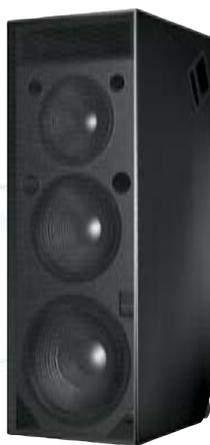
Meyer Sound's patented MTS-4A is a self-powered, four-way loudspeaker system uniquely capable of producing very high sound levels across the full audio range, including lower fundamentals and subharmonics. Powerful, yet relatively compact at 17 cubic feet, the MTS-4A offers an integrated solution for many applications — often eliminating the need for subwoofers and associated electronics.
