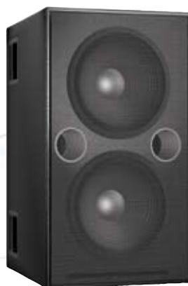
The PSW-2 high-power subwoofer is a self-powered, biamplified, fourth order bass-reflex subwoofer that is capable of being flown. The cabinet dimensions are identical to those of the MSL-4, allowing seamless integration into MSL-4-based arrays.
